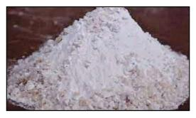
Customizable to client specifications, we also manufacture Ramming Mass for Chinese furnaces with a guarantee of higher life and consistent performance.
